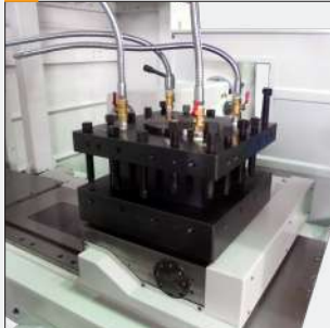
13 Hydraulic 4-Way Toolpost (Taiwan)
